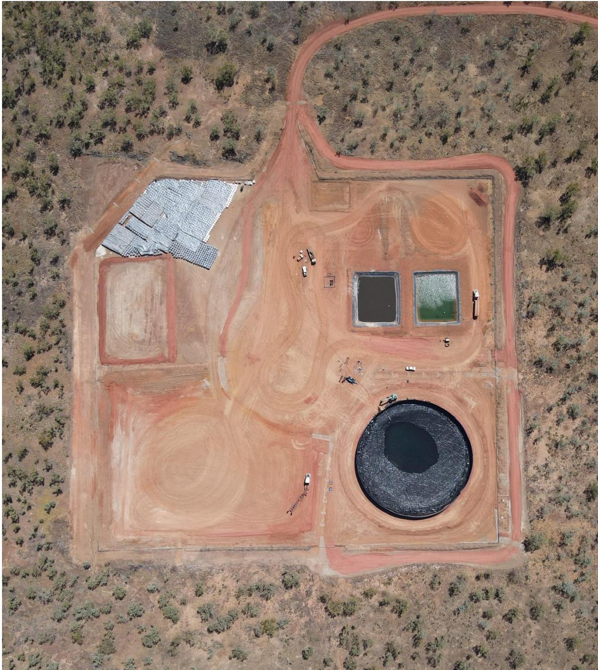
C-2H well pad with stimulation fluid tank installed
