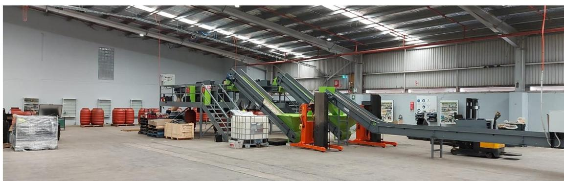
Battery sorting equipment operated by Envirostream in Melbourne, Australia.
