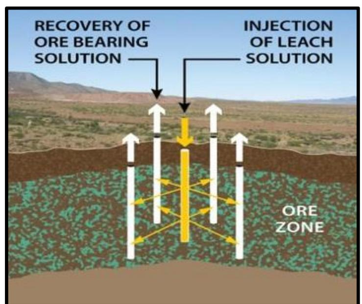
Figure 2. Schematic of In Situ Recovery process
