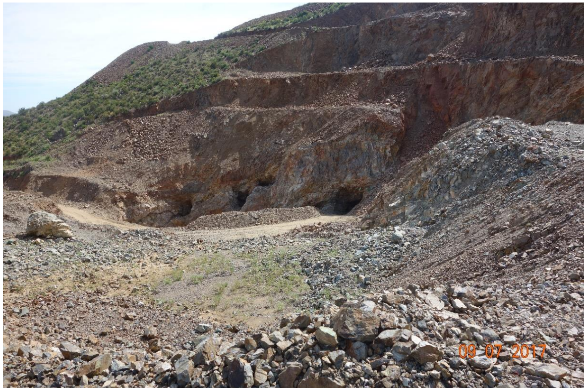
Fig 1. Historic copper-cobalt working, southern part of the La Cobaltera Exploration Licenses showing shearing and secondary copper minerals
