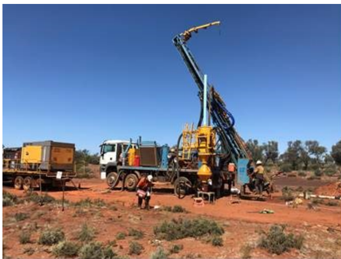
Figure 1 RC Drilling Underway at Saturn Metals' Apollo Hill Prospect – 19 March 2018.
