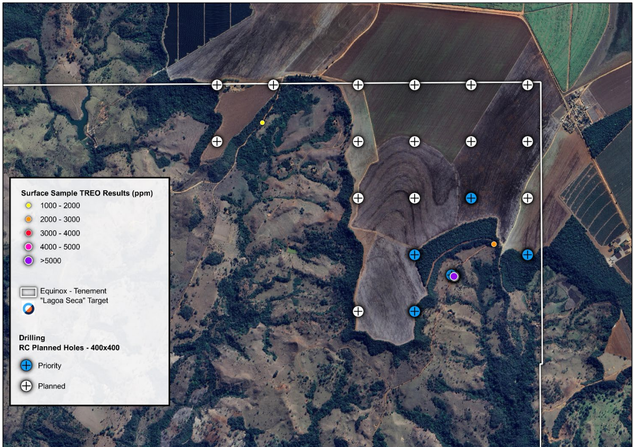
Figure 5: Proposed Drill Plan for Chumbo Prospect – Lagoa Seca Target.
