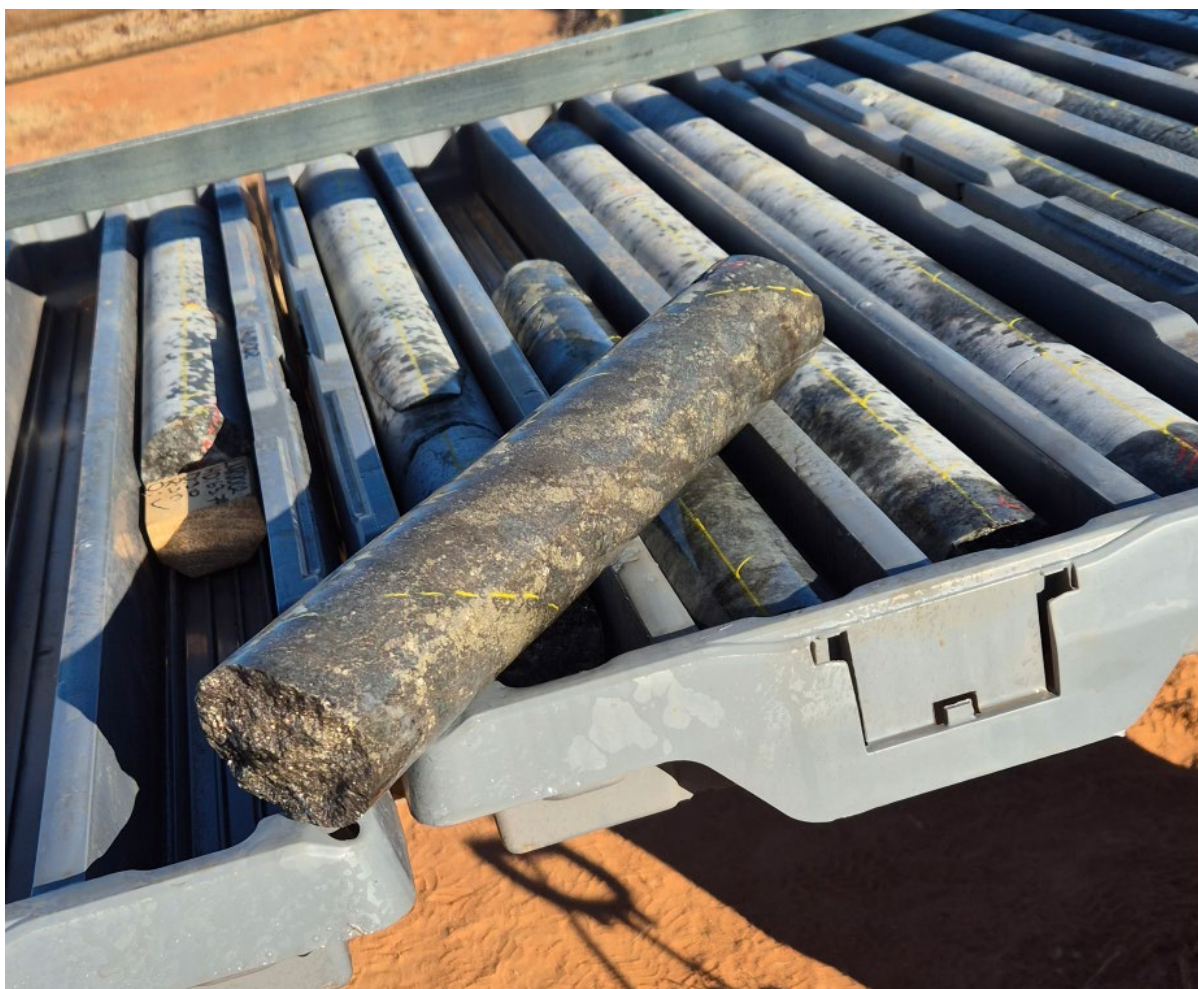
Figure 1 – LMRD002 showing visual semi-massive to massive sulphides from 61.2m to 62.m assay results for the interval can be found in the appendix.
