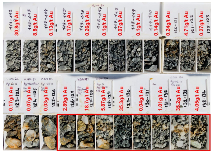
Figure 3 – RC drill chips – AHRC0330, 8m @ 12.9g/t Au intersection illustrated by red box outline and assays listed on chip tray – veining, alteration and sulphides noted in association with gold results. Broader intersection pictured - 14m @ 7.75g/t Au from 111m.
