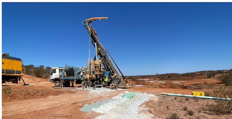
Plate 1 RC drilling underway at Apollo Hill Hanging-walls.
