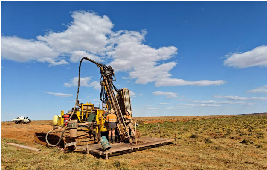
Plate 1 – Track mounted lake AC rig pictured 5km North of Apollo Hill in flat salt lake bed terrain – 10 September 2024.
