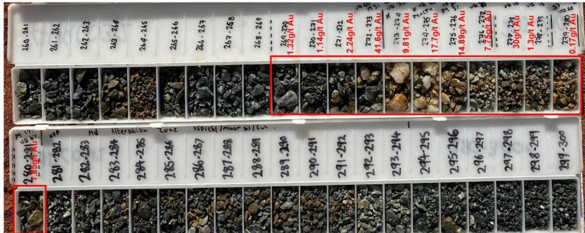
Figure 2 – RC drill chips – AHRC0312, 12m @ 9.98g/t Au intersection illustrated by red box outline and assays listed on chip tray – veining, alteration and sulphides noted in association with gold results.
