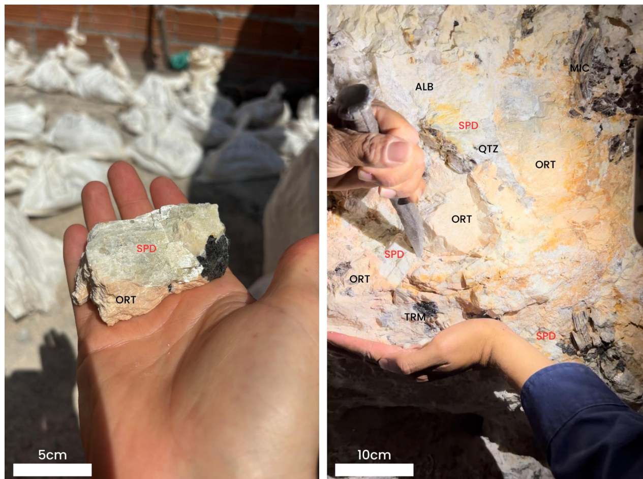
Figure 4: Spodumene-bearing rock chip sample (left) and in-situ spodumene (SPD) pegmatite with Orthoclase (ORT), Albite (ALB), Quartz (QTZ), and Tourmaline (TRM) in artisanal tunnel (right), located in License 830167/2013. 1
