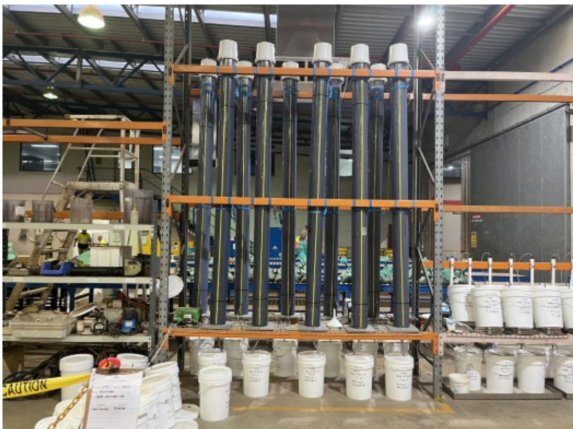
Plate 1 – Column Leach test work towards optimising gold recovery on Apollo Hill mineralised samples.
