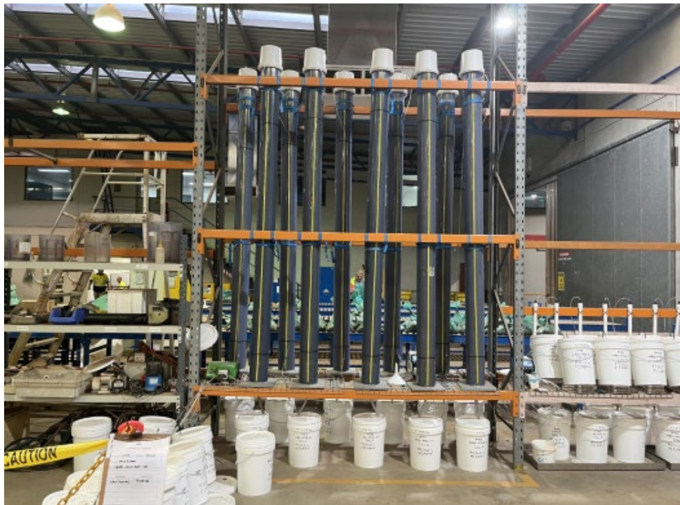
Plate 3 – Column Leach test work towards optimising gold recovery on Apollo Hill mineralised samples; columns due for completion in late April.
