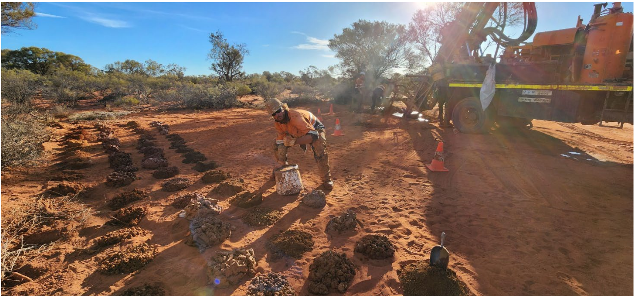
Plate 2 – AC Drilling in Progress – March 2023 – targeting hidden gold mineralisation under cover in greenfield terrains.
