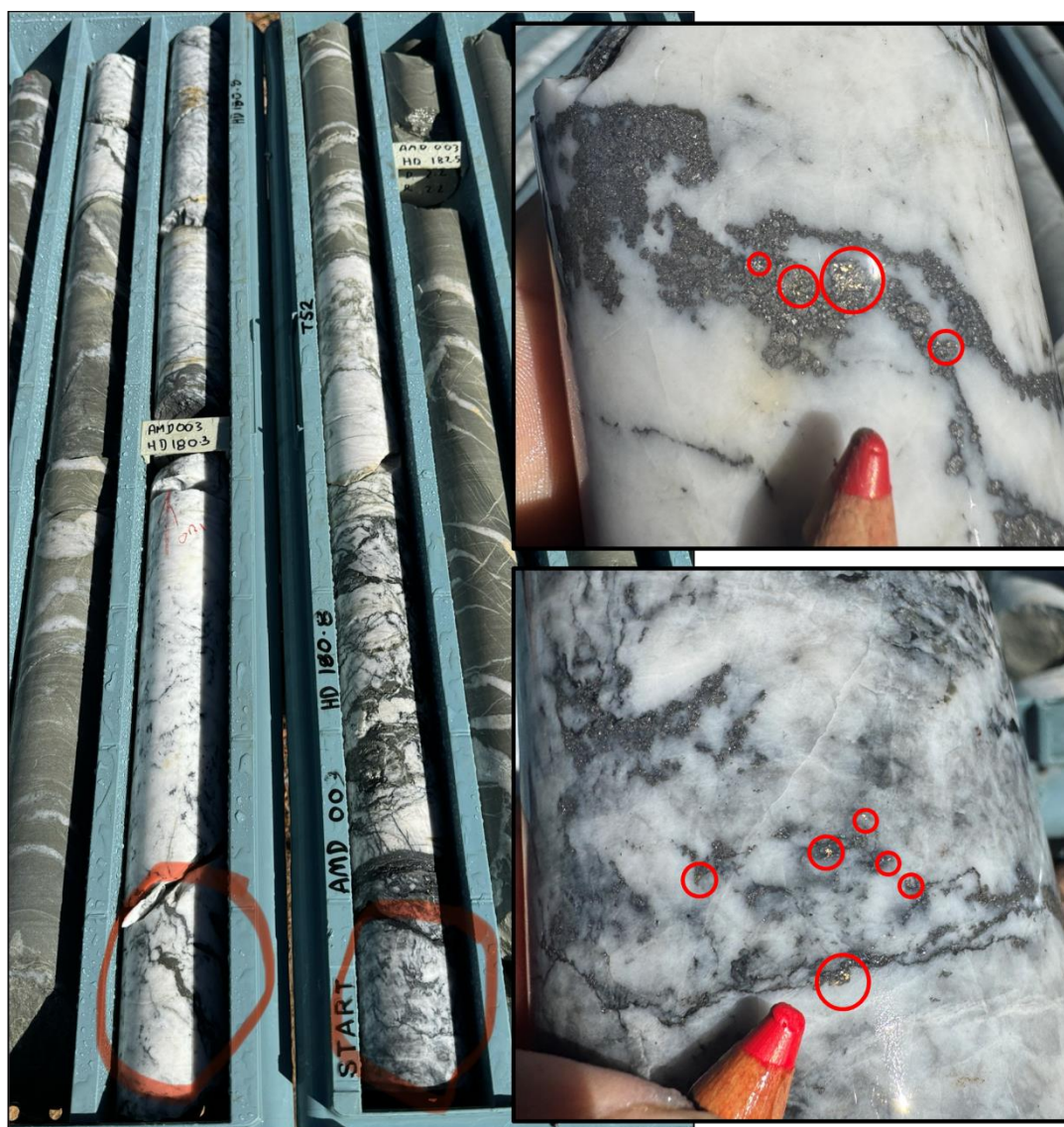
Figure 7. Composite image of a gold-bearing laminated quartz vein (left) from AMD003 , with close-up images highlighting the visible gold 2 at 180.0 metres down hole (top right) and 180.9 metres down hole (bottom right). Assays for this hole are currently pending.
