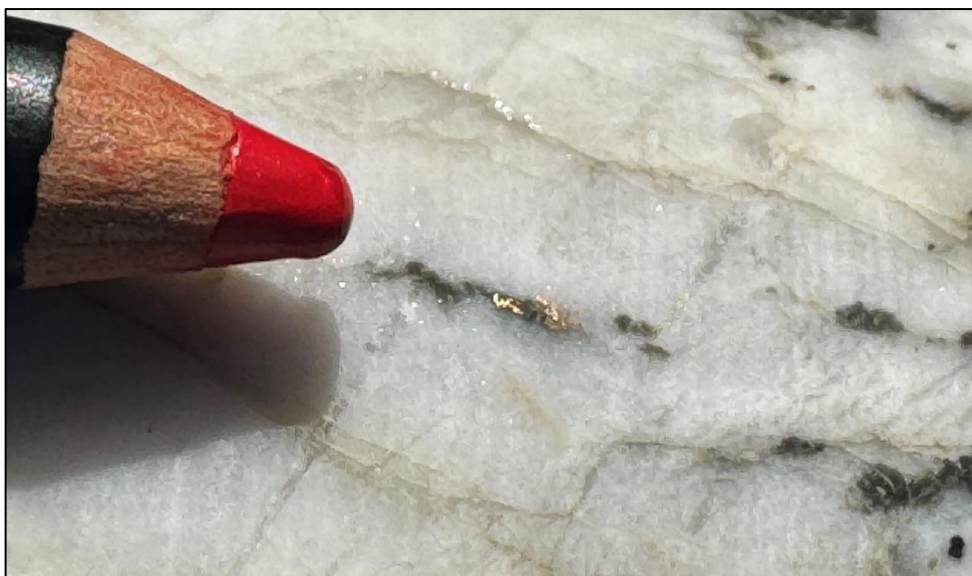
Figure 6. Visible gold 2 associated with a small chlorite veinlet in AMD003 at 159.5 metres down hole. Assays for this hole are currently pending.
