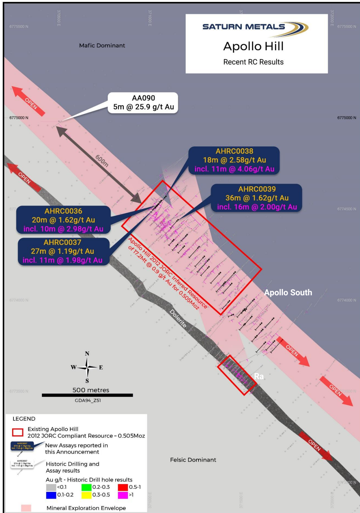
Figure 2. Apollo Hill phase 2 RC program in plan view showing recent significant assay results, historical drill results and Apollo Hill JORC 2012 compliant resource outline 1 .
