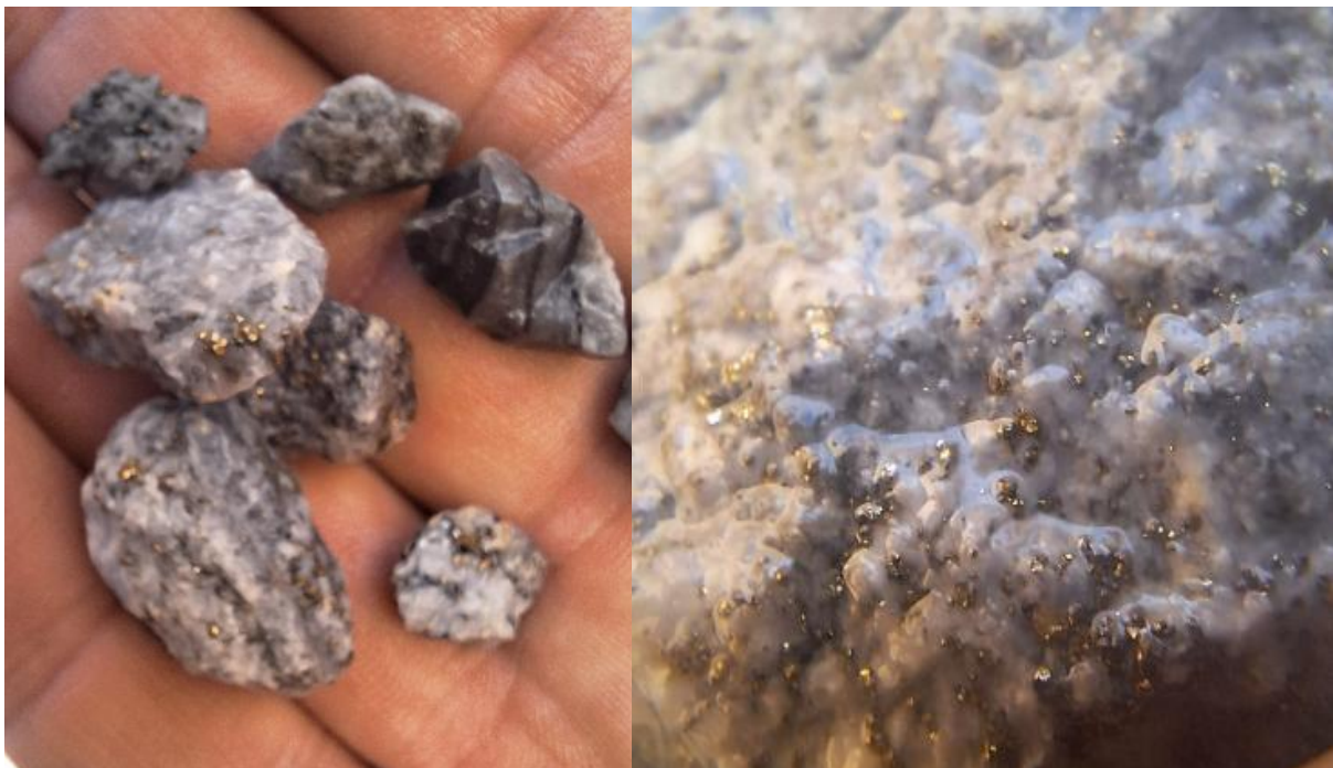
Figure 5: Sulphide metal mineralisation in the greywacke in the bedrock at Ibel South.
