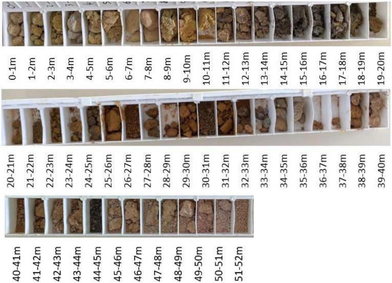
**Figure 3:** ASQ Aircore Drillhole SS001 Chip Trays
