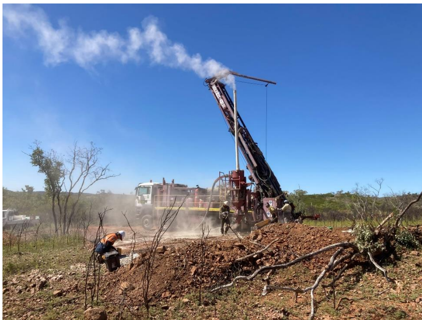
Plate 1: RC Drilling at King Solomon Prospect May 2022
