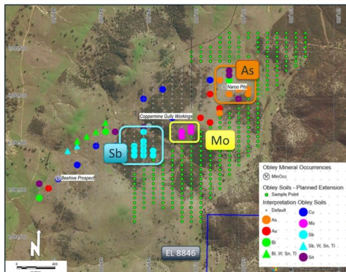
Figure 3: Obley Project – Soil Sampling Results (Source PBL 17<sup>th</sup> January 2022)
