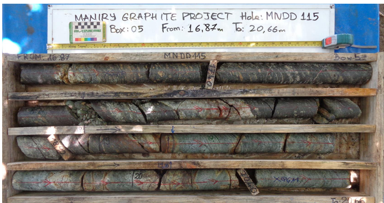
Fig 1: Example of oxidised grey graphite schist (16.87m-19.2m) and greyish-green granulite (code XGGM) in drill core from hole MNDD115
