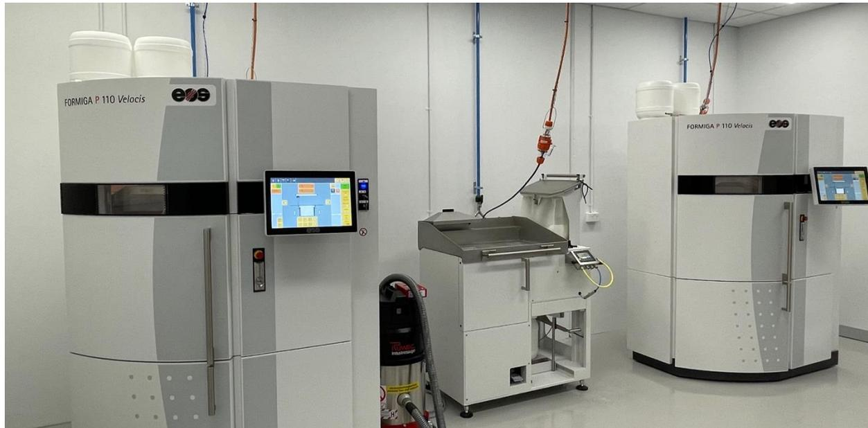
*Figure 2: Site fit out includes a large cleanroom and bio-model manufacturing space using polymer 3D printers.*
