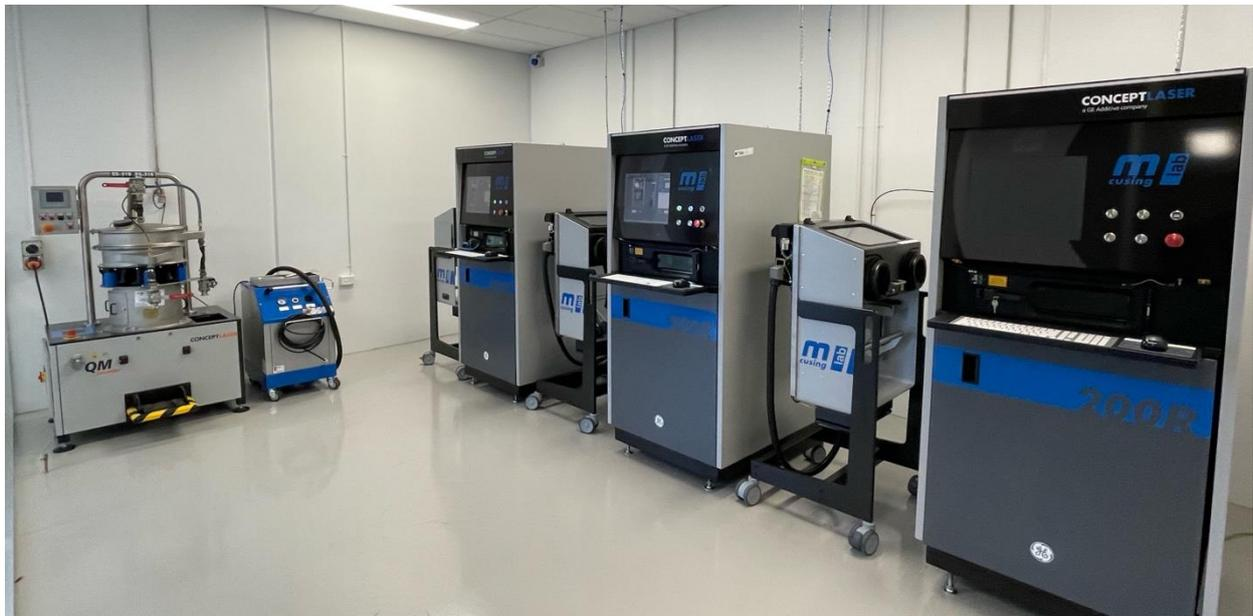
Figure 1: Three Titanium 3D printers installed at AAE Medical Manufacturing facility in Melbourne
