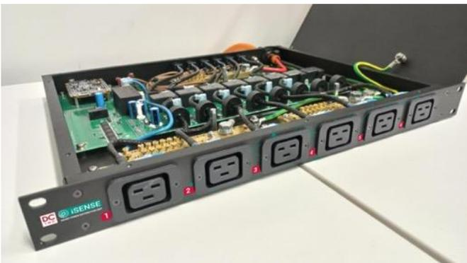
DC Two’s in-house developed PDU unit
