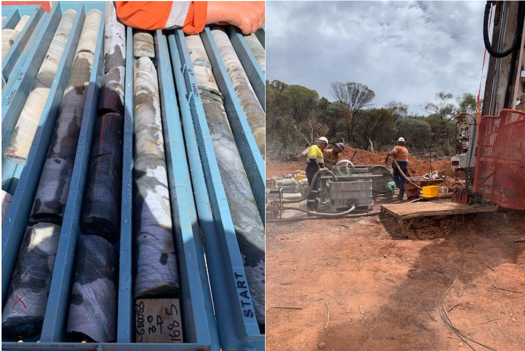
Figure 2: Diamond drill core from the footwall of Moonshine North and drill crew on site, October 2021.
