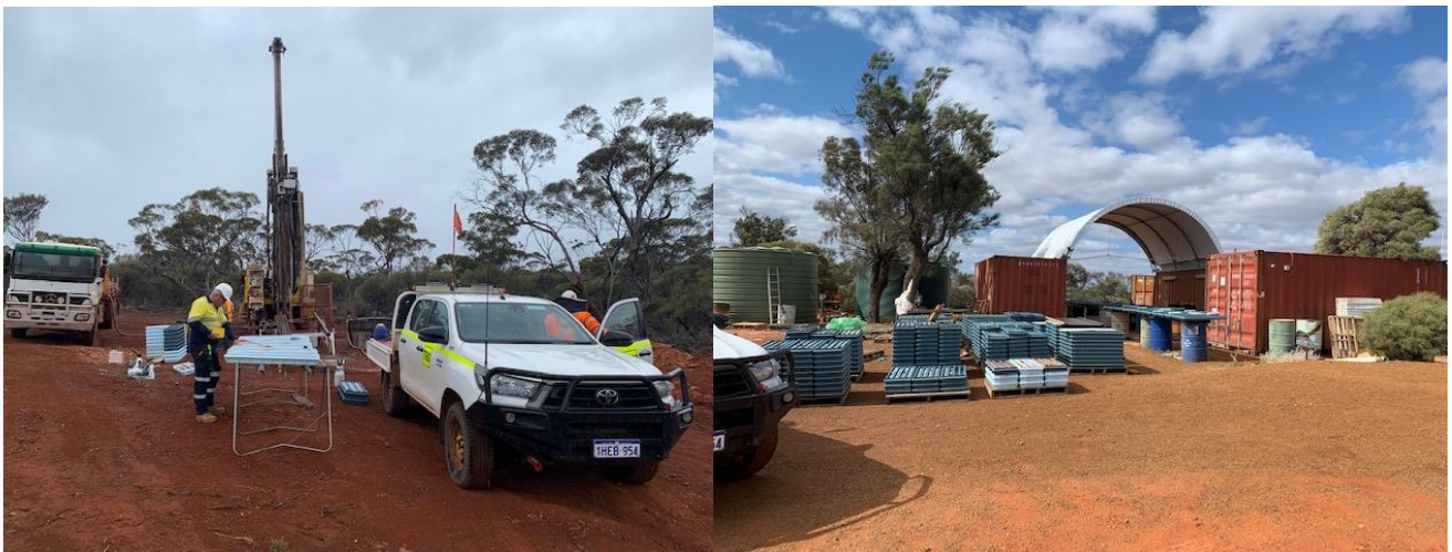
Figure 1: Drill team and geologists on site at Lake Giles at the conclusion of the geotechnical drilling programme of works in October 2021 and core trays stacked and ready for transport to laboratory for analysis.
