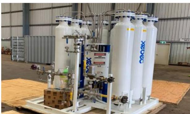
*Hydrogen Pressure Swing Adsorption*
