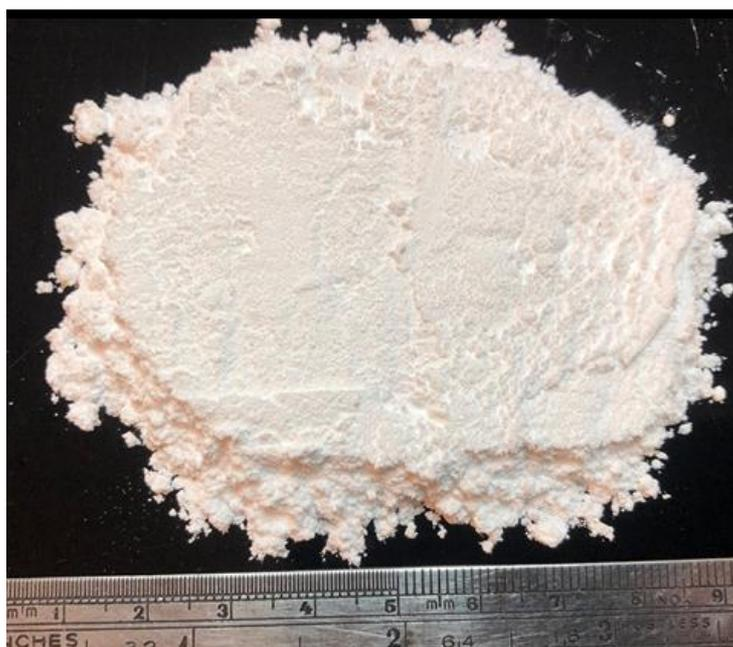
**Batch 7 HPA powder product (>99.99% purity) produced from an industrial chemical feedstock**
