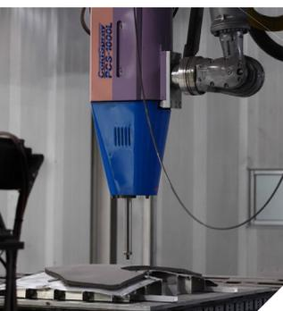
Illustration: Titomic's TKF 9000 creates an Invar tool for composites manufacturing.
