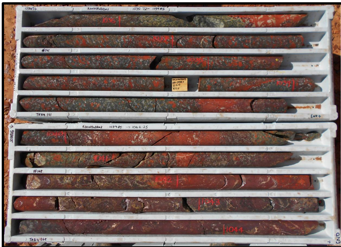
Figure 3: COHWDD03 from 1035.72-1044.25m exhibiting strong haematite-sericite alteration within brecciated Donington Granite.
