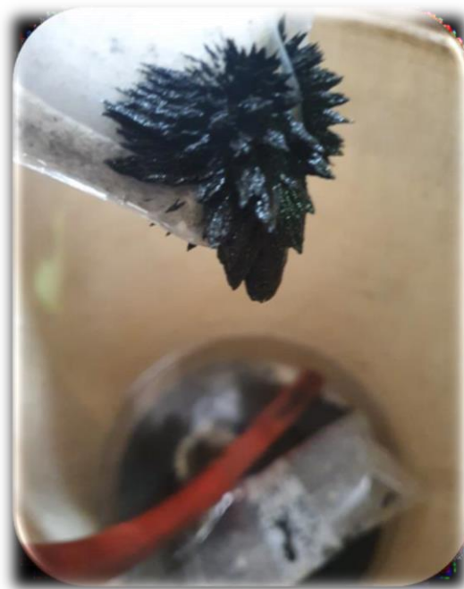
Figure 3: Magnetic Concentrate - Magnetic particles attracted to a hand magnet from the upper saprolite table concentrate 1
