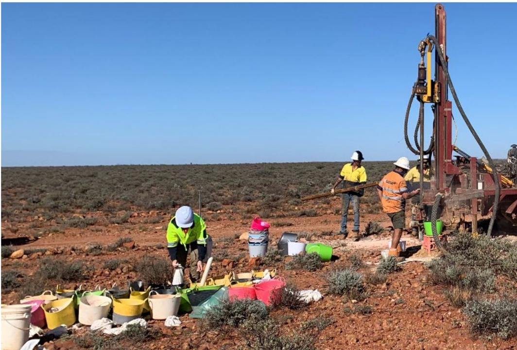
*Photo Air Core Drilling Operations at Comet*
