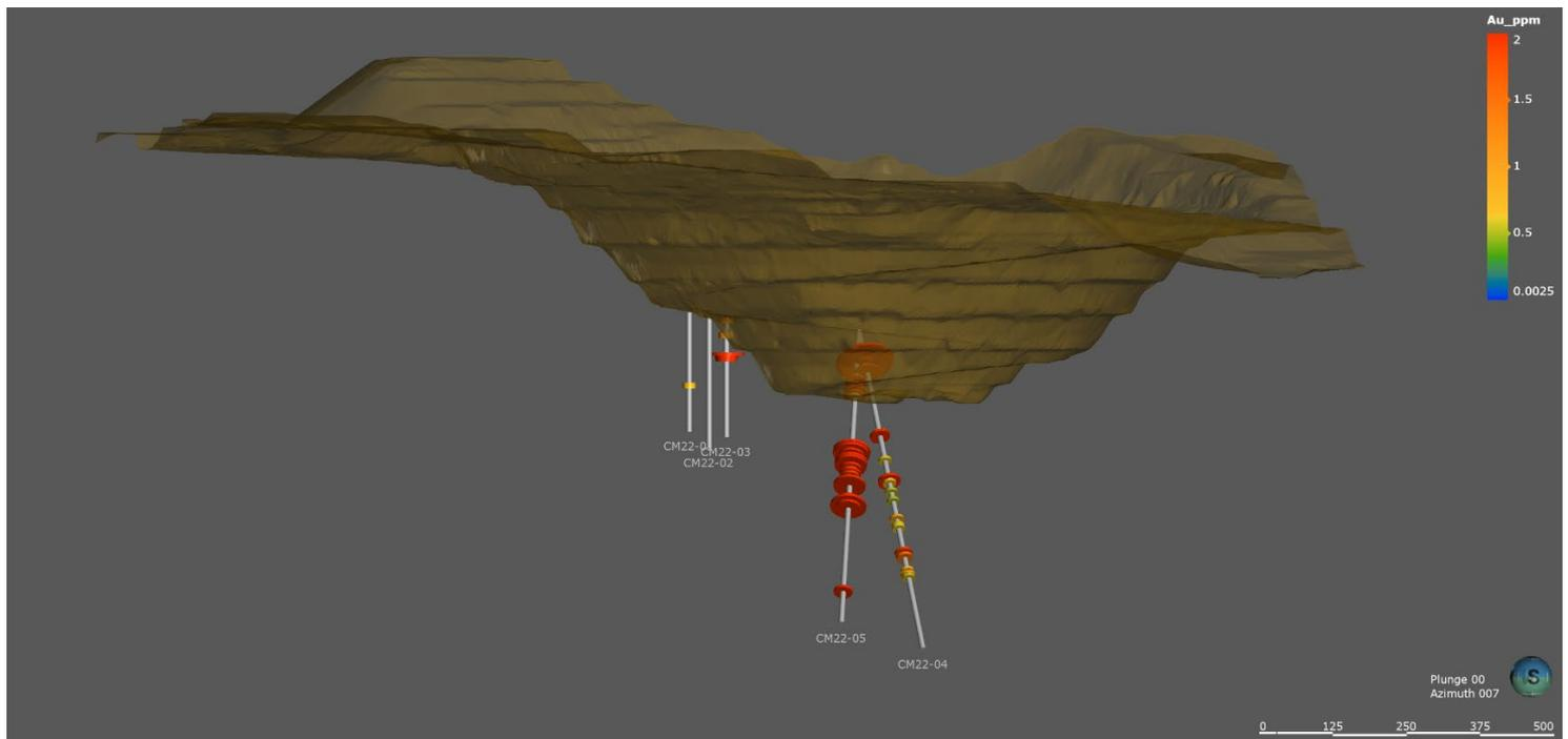
Figure 1: Cross Section of the five completed drill holes with assay results. View looking north, Azimuth 005
