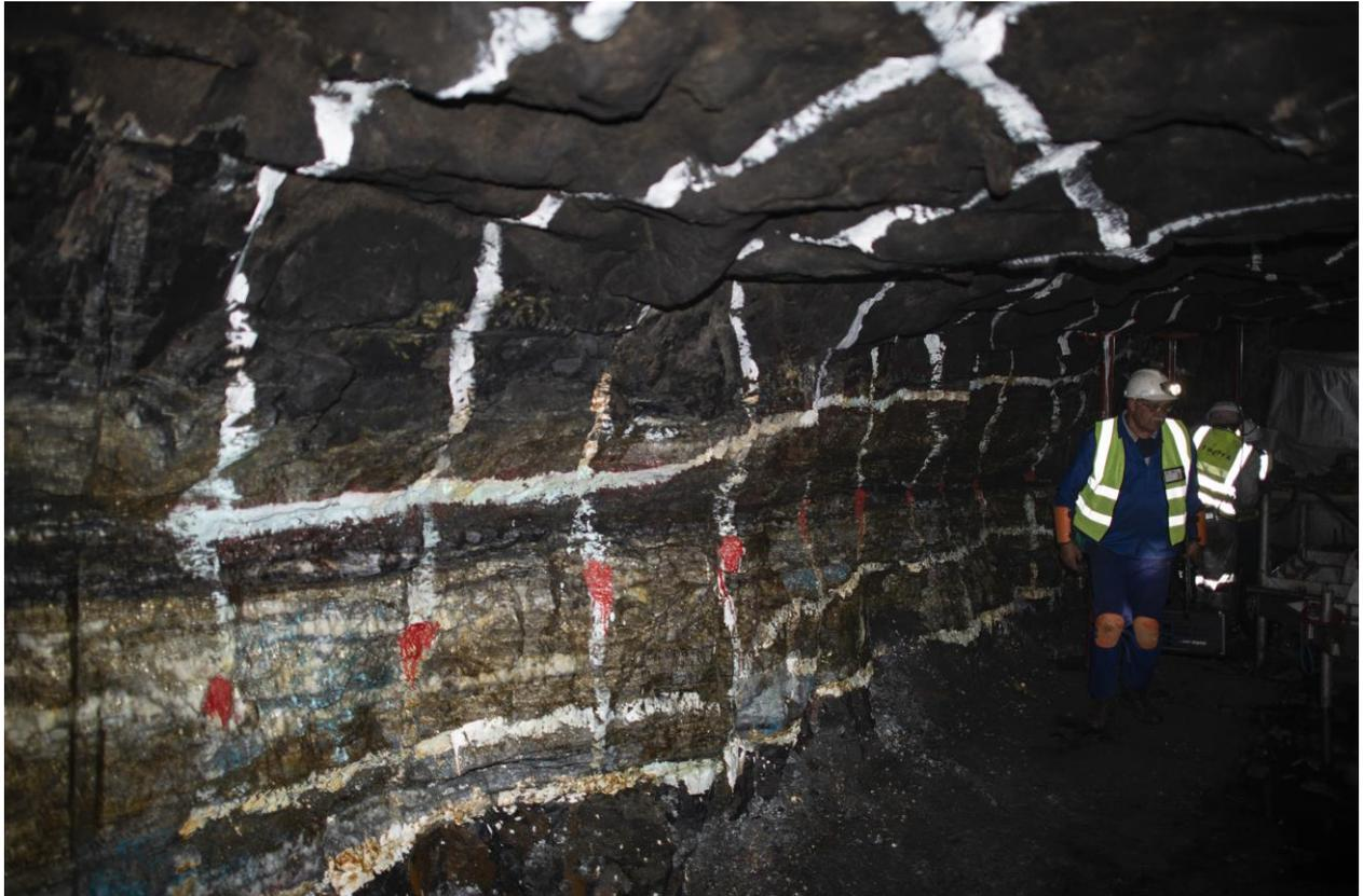
**Figure 2: Gold reefs being marked up to for trial mining**
